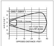
**SBEF & SBRF1:** use with individual glass fiber optic assemblies in lieu of model SBF1 where it is inconvenient to run fibers from a single scanner block.
